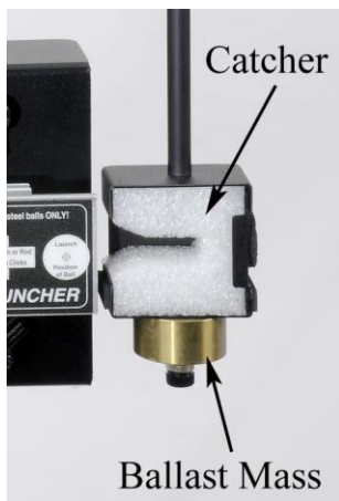
Figure 5: Ballast mass and pendulum alignment.
