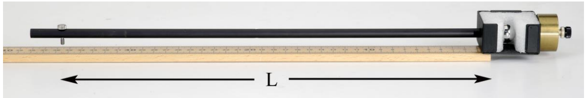
Figure 6: Finding the center of mass to find the length of the pendulum.
